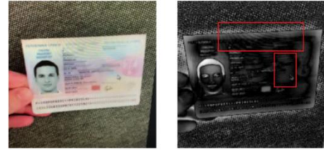
Figure 2. Screen stripe patterns enhanced using a high-pass frequency filter with a mask radius of 8
