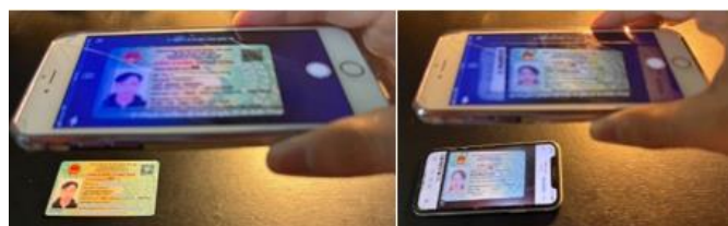
Figure 1. Example of the electronic identity verification process with a genuine ID card (left) and a spoofed ID card (right)
