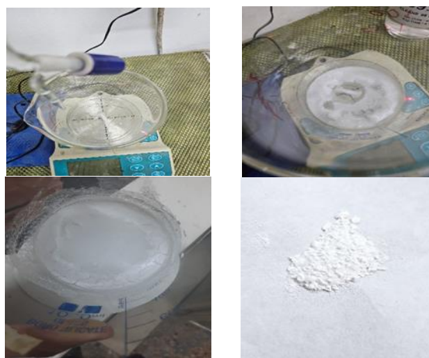
Figure 2. Preparation steps of NanoSiO 2
