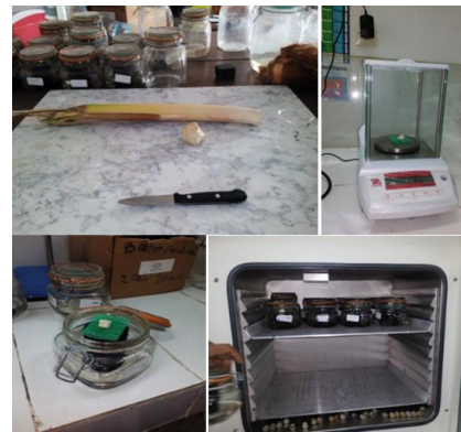
Figure 2. Sample preparation for the study of sorption isotherms
