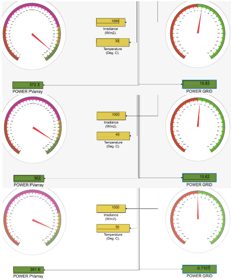
Figure 12. Sharing PV array and grid to supply the load under step change in temperature with constant irradiance
