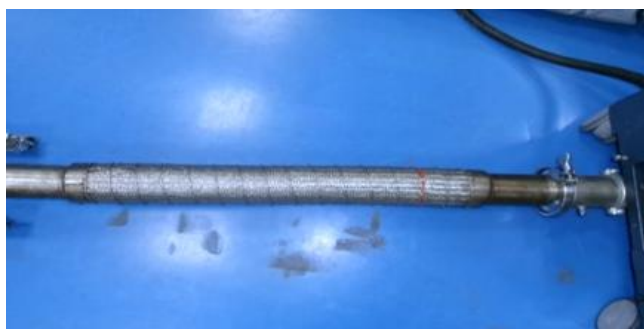
Figure 8. Sampling pipe without heating and insulation
