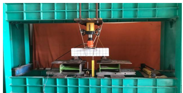
Figure 11. Geopolymer mortar flexural strength testing
