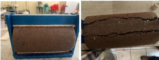
Figure 15. Geopolymer mortar split tensile strength testing
