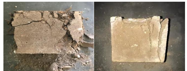
Figure 9. Visual appearance of geopolymer specimens after compressive strength test
