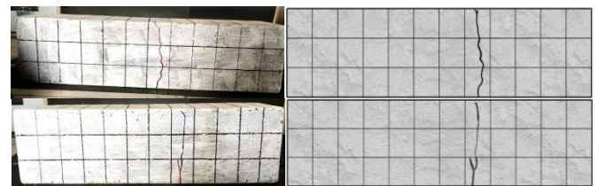
Figure 13. Visual appearance of geopolymer specimens after compressive flexural strength testing
