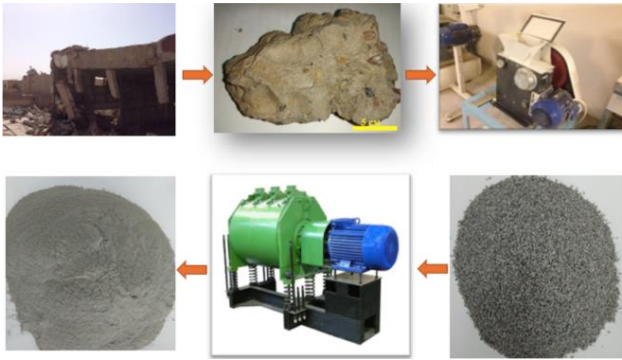
Figure 1. Procedures of binder preparation
