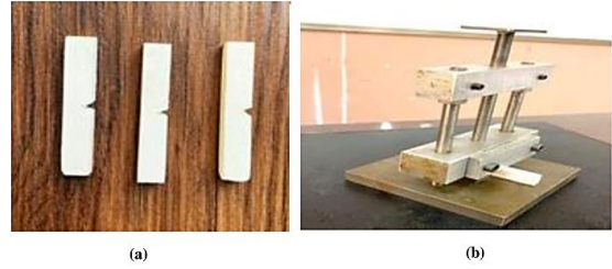
Figure 4. Pictures of (a): SENB samples, (b): The method of creating a crack within fracture toughness (SENB)
