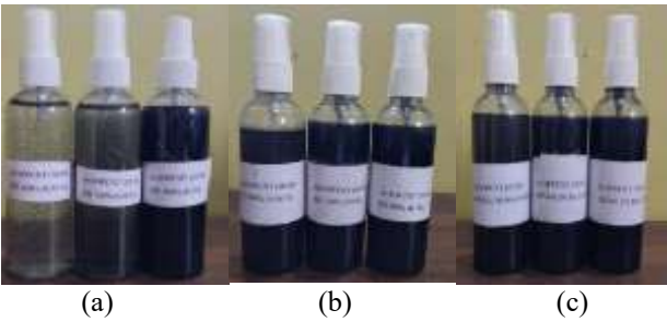
Figure 2. Prepared graphene-MWCNT/distilled water, ethylene glycol and DW-EG(70:30) samples
