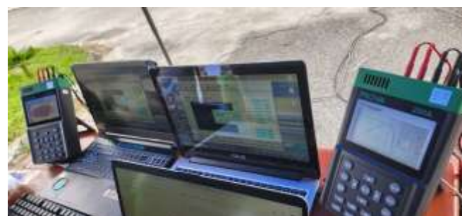
Figure 7. A module analyzer and a data logger for data collection
