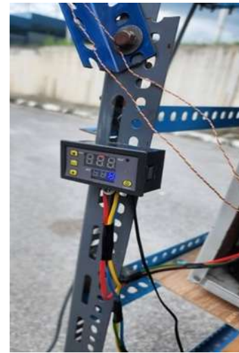
Figure 8. Thermostat-controlled chiller system to fix the inlet temperature
