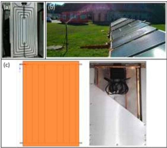
Figure 1. The various types of PV/T systems (a) PV/T cooling with split flow absorber design [13]; (b) Water cooling by sprinkling on the PV plate; (c) Effect of water-cooling using copper pipe [14]
