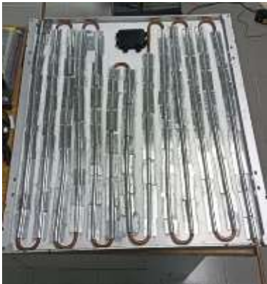
Figure 2. PV/T systems with a copper tube at the back of the absorber
