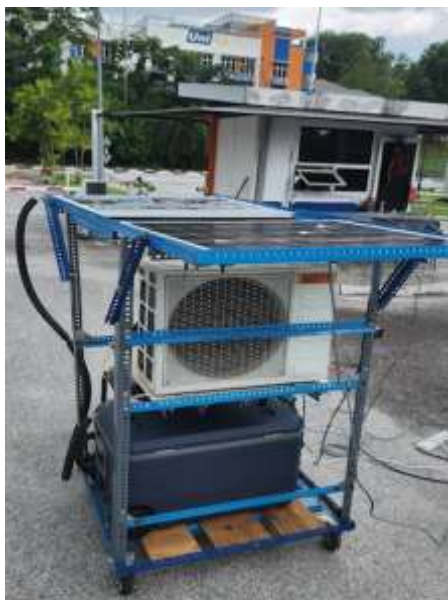
Figure 5. The PV/T water-cooling setup
