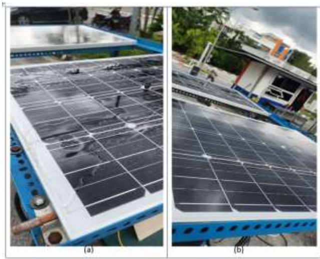
Figure 9. The PV/T and PV systems: (a) PV/T cooling with spiral flow absorber design, (b) Standard PV module
