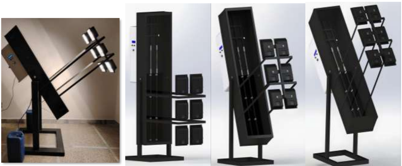
Figure 2. Experimental set-up of the thermosiphon heat pipe flat plate collector presents the three angles of inclinations
