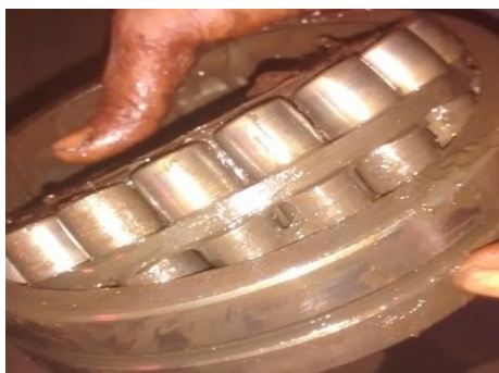
(a) Damaged pump DE bearing
