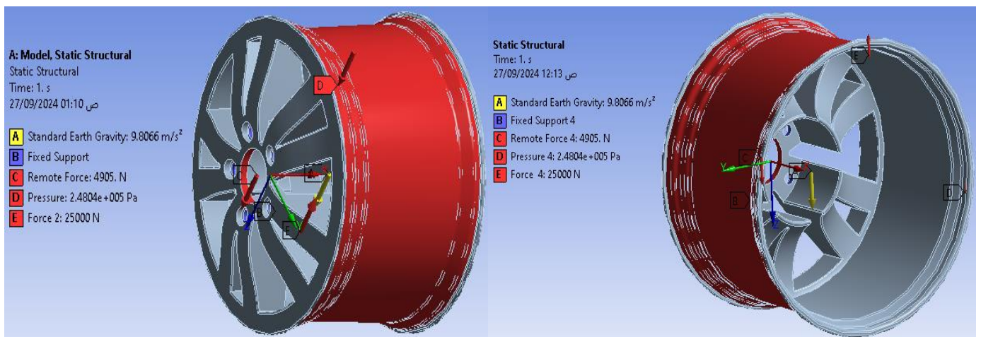
Figure 3. Type of force applied, its magnitude, and where it affects the wheel
