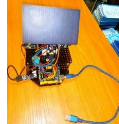
Figure 14. Prototype of the designed solar tracking system
