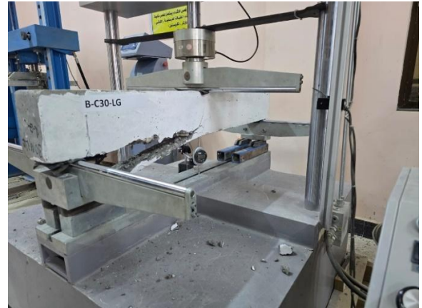
Figure 12. Failure mode for B-C30-LG
