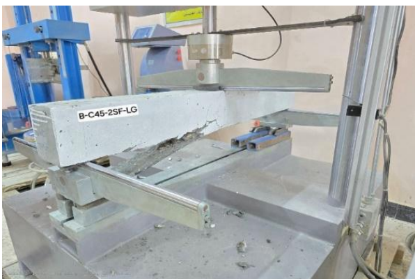
Figure 22. Failure mode for B-C45-2SF-LG
