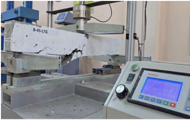
Figure 20. Failure mode for B-C45-LTG
