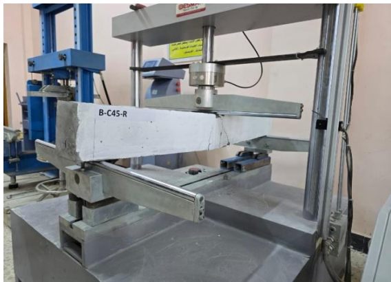
Figure 10. Failure mode for B-C45-R
