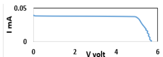
Figure 9. Photovoltaic I-V characteristics of red cabbage dye and ZnO nanoparticles sensitized solar cell
