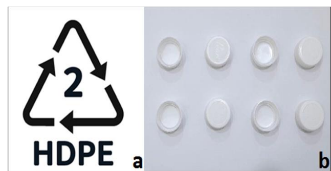
Figure 3. (a) Recycling symbol indicating high-density polyethylene (HDPE); (b) HDPE bottle caps collected from discarded PET bottles, utilized as a secondary reinforcement component
