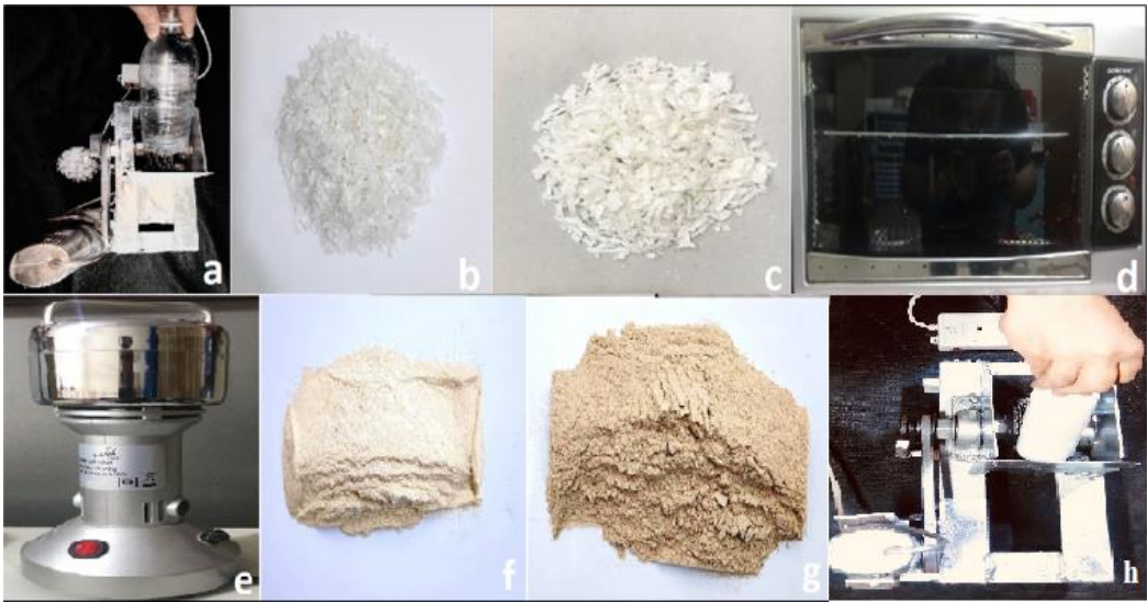
Figure 4. Stages of preparation of PET and HDPE reinforcing materials: (a) Locally fabricated cutting machine used for initial shredding of plastic bottles PET; (b) PET fragments after cutting; (c) HDPE fragments after cutting; (d) Electric furnace used for melting PET (at 250°C) and HDPE (at 135°C); (e) Grinding machine used to pulverize the cooled melted materials; (f) PET granules after grinding (particle size ≈ 53 μm); and (g) HDPE granules after grinding (particle size ≈ 53 μm); (h) Locally fabricated cutting machine used for initial shredding of plastic bottles caps HDPE or another HDPE
