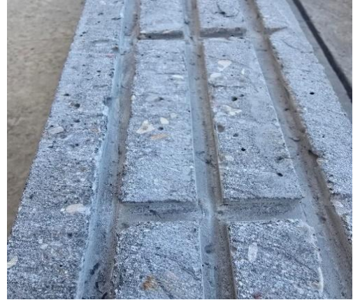
Figure 5. Preparing specimen grooves for subsequent application of CFRP
