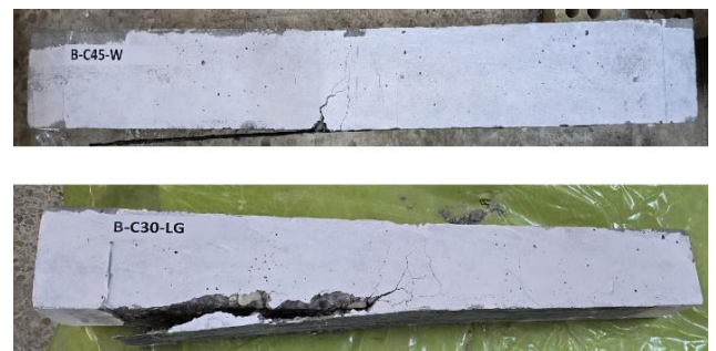
Figure 29. Various modes of failure, here for B-C45-W and B-C30-LG
