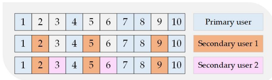
Figure 7. Detailed breakdown of sub-band allocation and channel filling process across time steps t and t + 1 , illustrating interference-free sharing
