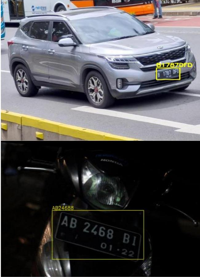
Figure 12. EasyOCR test results with the proposed method
