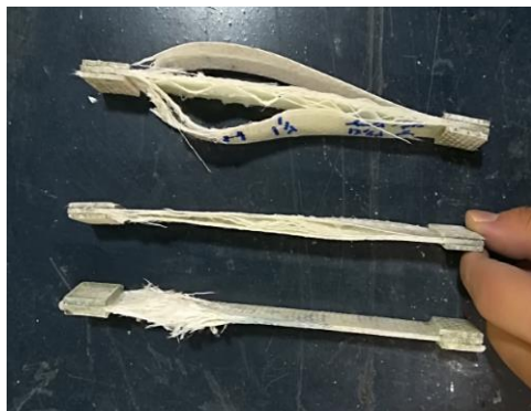
Note: upper - hand layup; middle - vacuum bag; lower - VIP
