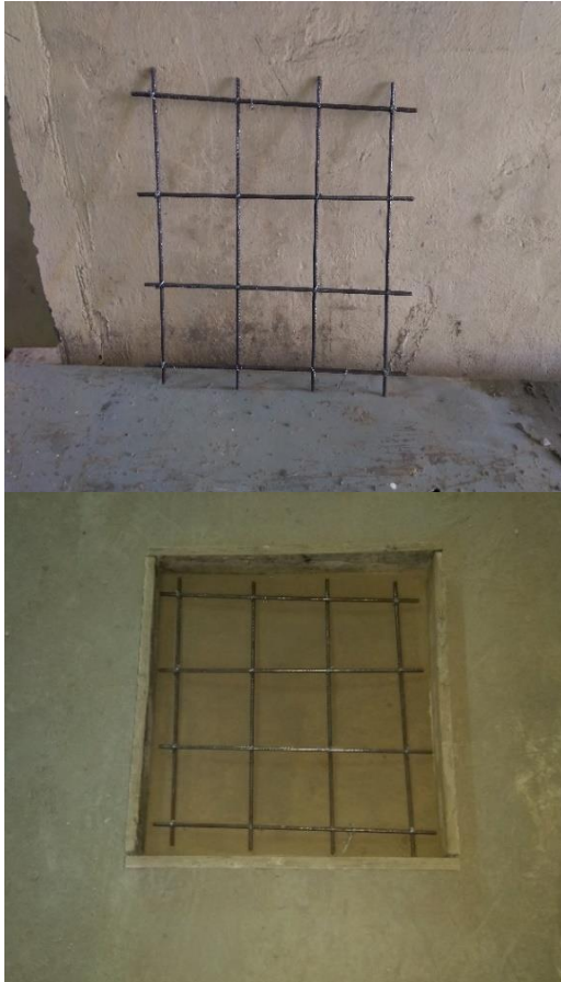
Figure 1. Details of reinforcing steel used in slab specimens
