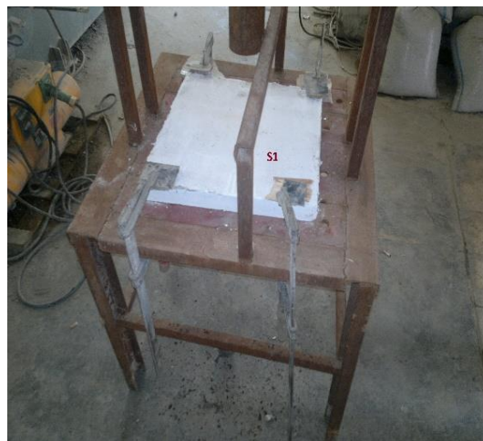
Figure 6. Specimens under impact test
