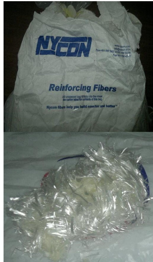
Figure 2. Package and appearance of nylon fibers used in slab specimens
