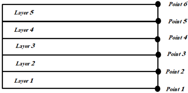
Figure 5. Number of layers and points along thickness of FG-plate
