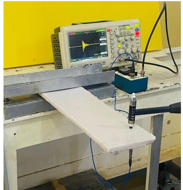
Figure 7. Vibration test machine of cantilever FG-plate
