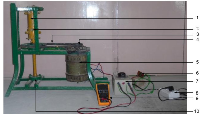
Note: 1- Mould, 2- Clamp, 3- Belt, 4-Pulley, 5-Motor, 6-Rectifier, 7-Variac, 8-Extension cord, 9-Multimeter, 10-Bearing
