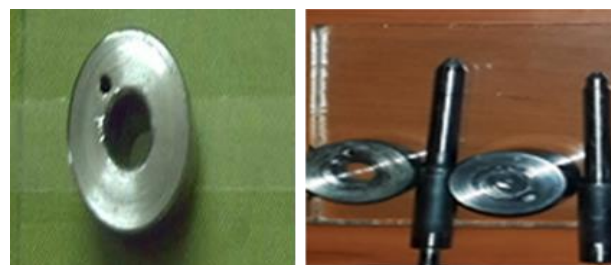
Figure 9. Molds utilized to generate special hardness analysis sample preparations
