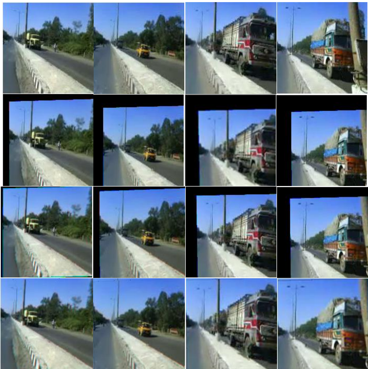
Figure 22. Results of the suggested stabilizing technique, broken down per stage for Highway Video 6 top row: Every 25 th frame of the original video sequence. Second row: estimated frames with large accumulation error. Third row: filtered video frame sequence. Last row: edge completed full frame stabilized video sequence
