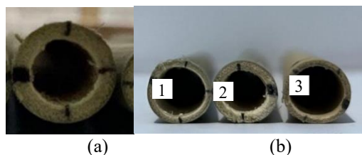
Figure 8. (a) bamboo diameter before drying (round-shaped); (b) diameter deformation in tamiang bamboo samples from (1) oven drying, (2) hot-steam air drying, and (3) air drying
