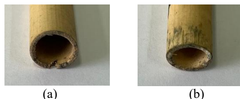
Figure 9. Damaged air-dried tamiang straws due to the attacks of: (a) powder beetles, (b) mold/fungus
