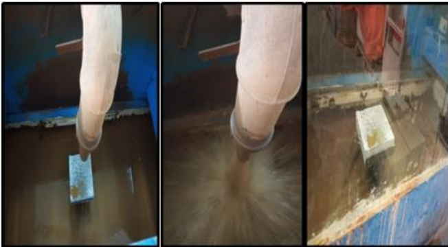
Figure 7. 0.6 mm distilled sand was used as graded sand
