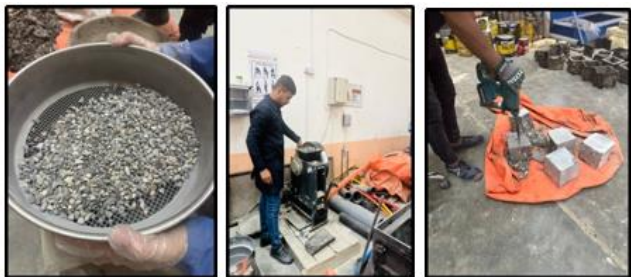
Figure 4. Crushing the concrete cubes, grinding them, and then sifting them through sieve No. (10)
