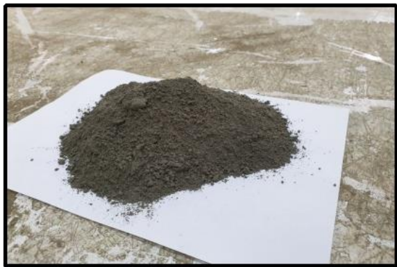
Figure 2. The sample of the Portland cement of the R42.5 type
