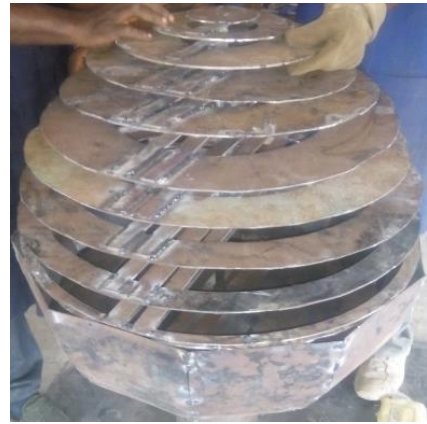
Figure 15. 10 section-sphere under development with lower hemisphere
