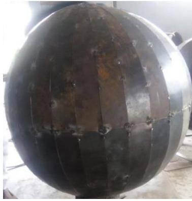
Figure 18. Complete 30-Section 225liter capacity spherical tank developed
