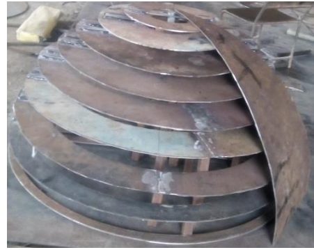
Figure 14. First section being welded to the upper hemisphere
