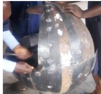
Figure 17. 30-Section 225 liter capacity spherical tank under development
