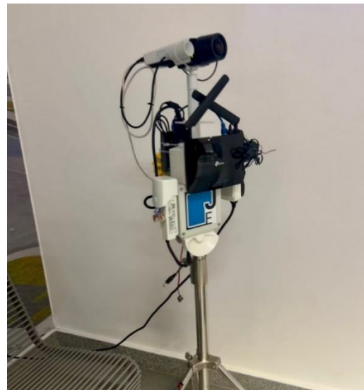
Figure 2. Tripod with SED sound event detector, security camera and communication infrastructure used in the experiment at Prague Airport
