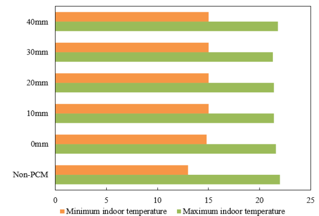
Figure 7. Indoor temperature variation under different thicknesses of PCMs in the east wall
