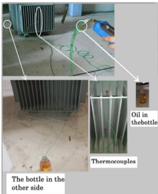
Figure 8. The experimental setup for the temperature rise measurement
