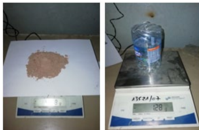
Figure 2. Weighing of date palm nut powder and epoxy resin
