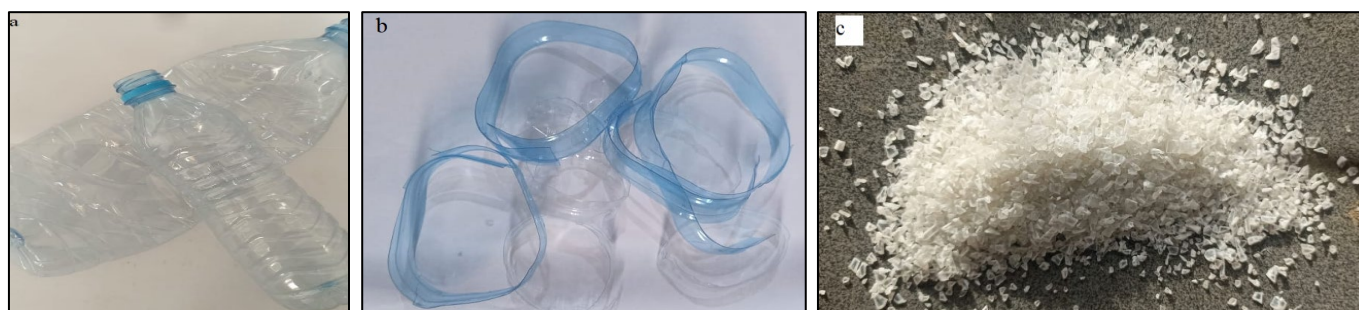
Figure 5. (a) The bottles waste; (b) The shredded bottles; (c) Particles PET ground to 1, 25mm
