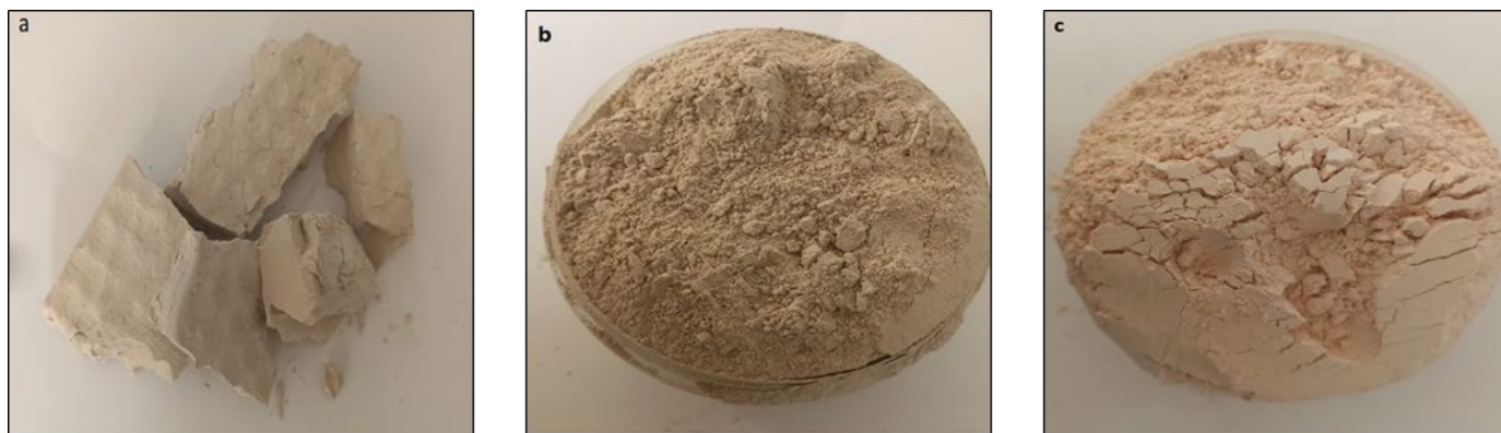
Figure 3. (a) Cake sludge; (b) Grinded cake sludge; (c) Grinded and calcined cake sludge
