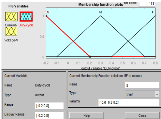
Figure 7. Membership function of output (duty-cycle)
