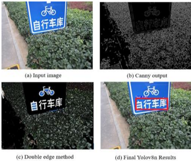
Figure 3. Input image, output of canny edge detection, double edge method and final Double Yolo approach
