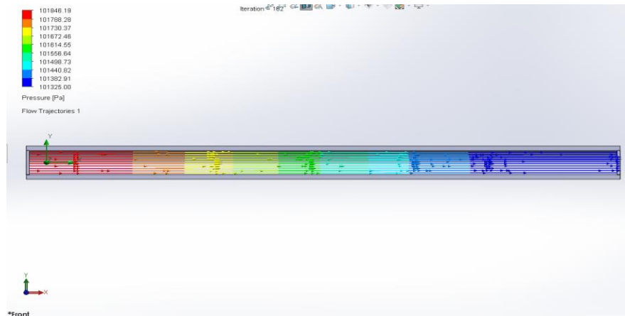
Figure 4. Pressure variation of 500 GPM flow through 6-inch MS pipe diameter
