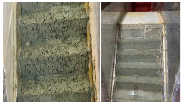
Figure 6. Normal and porous concrete steps of the stepped spillway model
