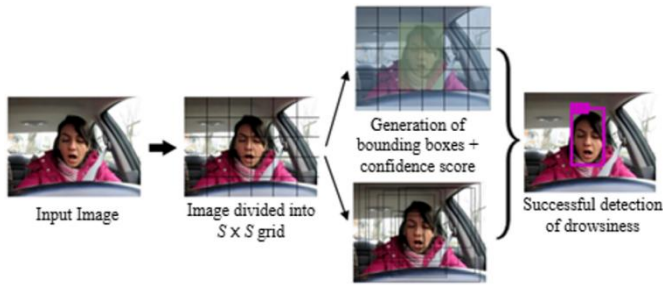
Figure 5. Consecutive phases of the YOLOv4 model were implemented to detect drowsiness
