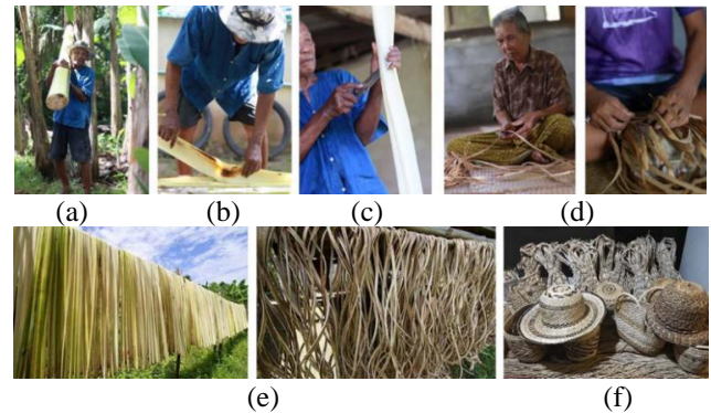
Figure 4. (a) Cutting; (b) Peeling; (c) Stripping; (d) Pressing and weaving; (e) Banana fiber before and after drying; (f) The existing banana fiber products
