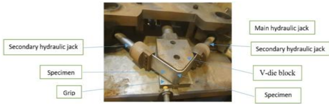
Figure 4. The test rig showing the use V-die shape (90°) in the stretch forming process
