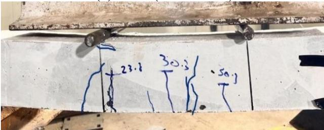
(c) SF 1.0 (Flexural failure)
