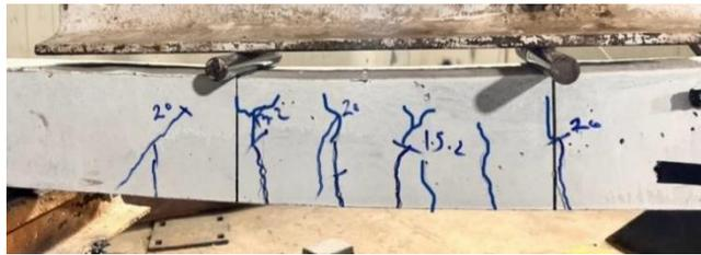
(a) SF 0 (Shear failure)
