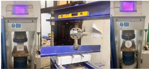
Figure 4. Test devices of cube, prism, and cylinder
