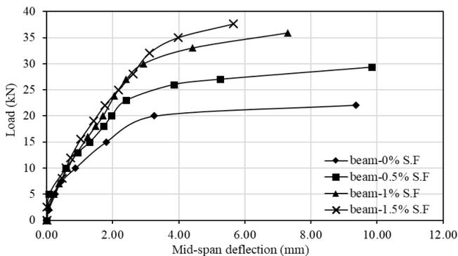
**Figure 8.** Load-deflection (beam with and without steel fibres)
