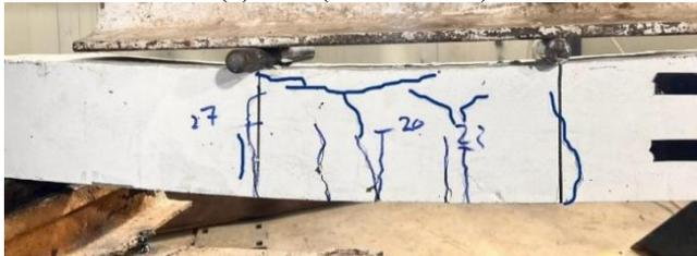
(b) SF 0.5 (Shear failure)
