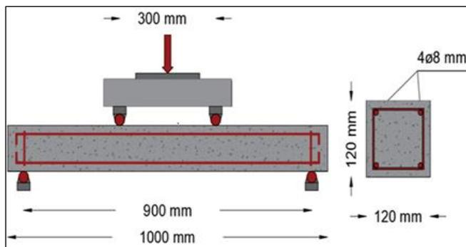
**Figure 1.** Details of RCB cross-section
