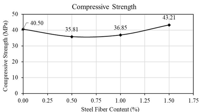
Figure 6. Steel fibre content influences on compressive strength
