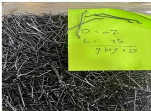
**Figure 2.** Physical characteristics of Hooked-end steel fibres
