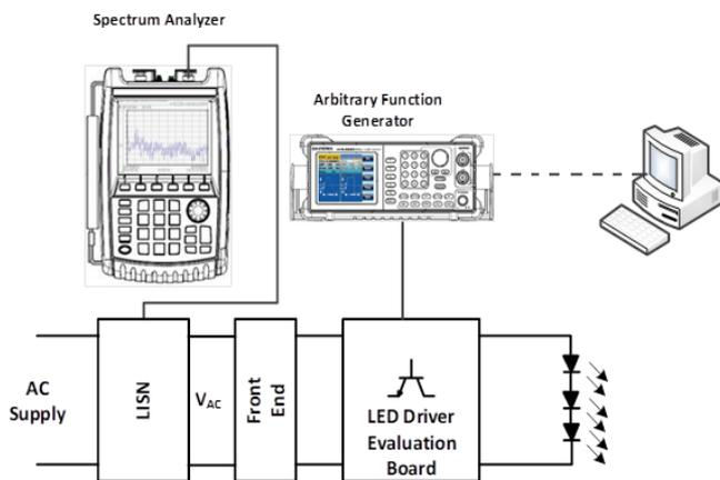
Figure 1. Conducted emission measurement setup
