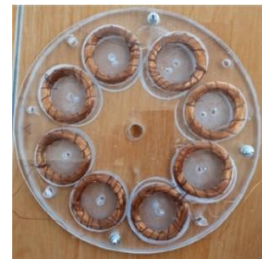
Figure 9. Stator disc with a number of 8-pole windings
