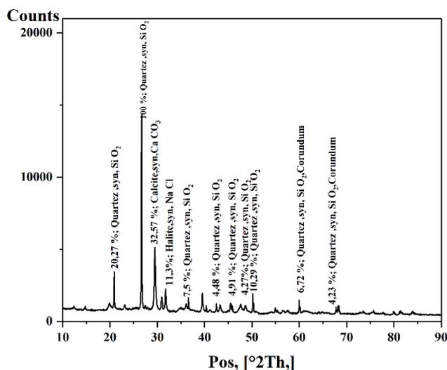
**Figure 7.** X-ray diffractogram of the studied clay
