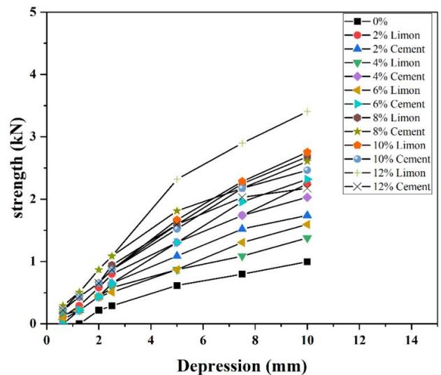
**Figure 10.** Effect of treatment on compressive strength
