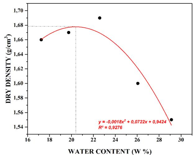
**Figure 6.** Compaction curve for Chott el Hodna clay
