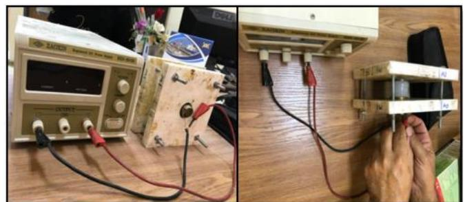
**Figure 5.** The thermal conductivity coefficient measuring device
