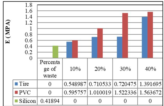
Figure 7. Calculation of elastic modulus E
