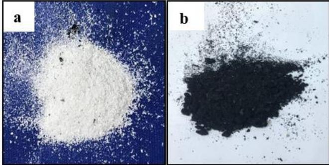
**Figure 3.** The powder (a) PVC, (b) Tire
