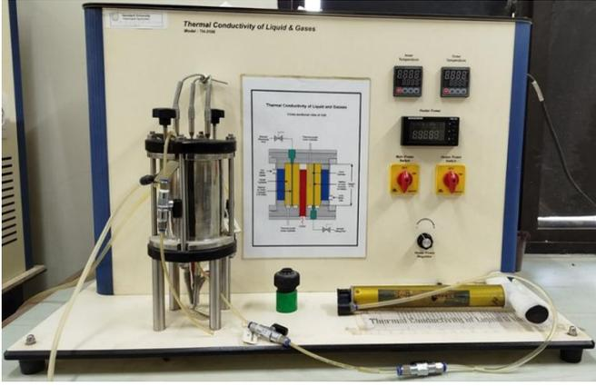
**Figure 5.** Thermal conductivity of liquid and gases
