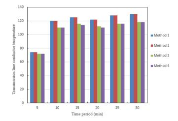
**Figure 5.** Conductor temperature calculation results of transmission line under freezing weather
