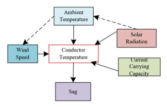
**Figure 1.** Factors affecting conductor temperature under freezing weather
