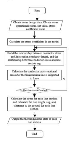
**Figure 4.** Accurate calculation process of the thermodynamic state of transmission line under freezing weather conditions
