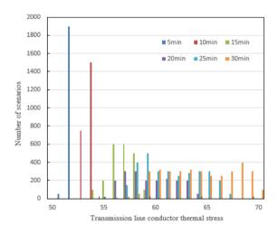
**Figure 9.** Thermal stress distribution of transmission line conductors at different time periods
