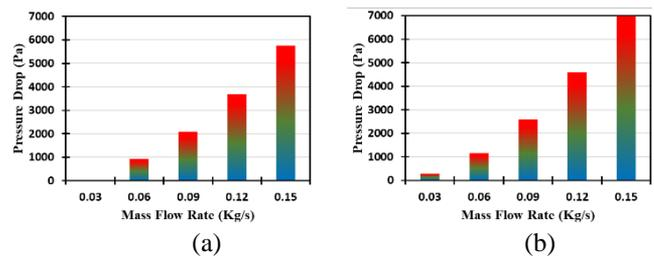
**Figure 17.** The simulation-based pressure drop bars across the inner tube of the HE under all working condition of variant mass flow rates: (a) Traditional, (b) Dimpled
