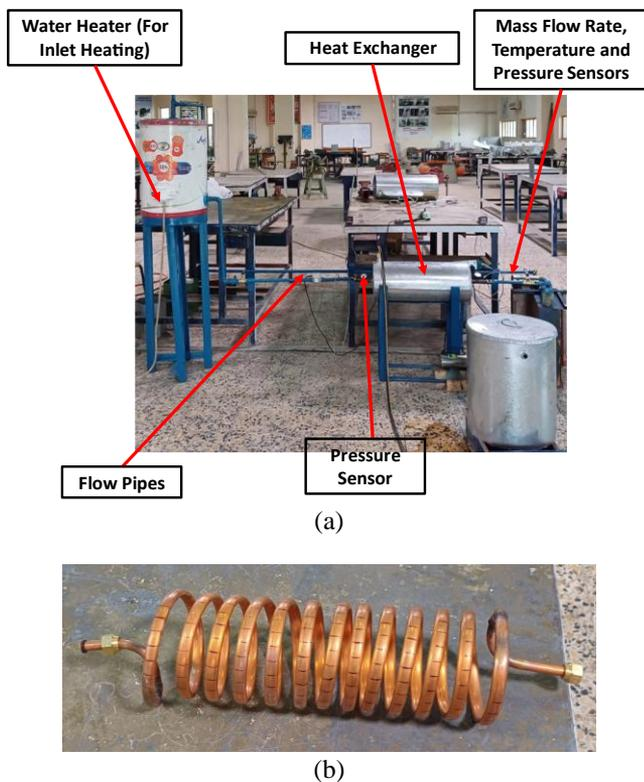
**Figure 10.** Experimental setup: (a) Test rig, (b) Helical tube
