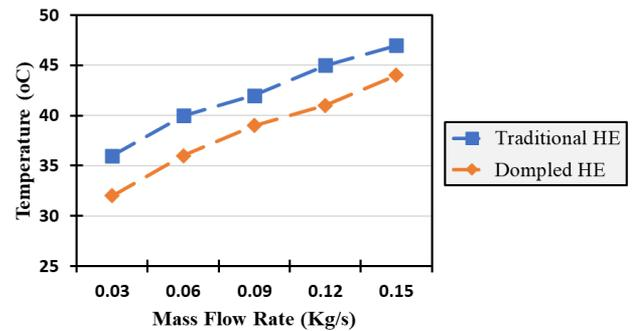
**Figure 19.** The experimental-based temperature recordings across the exit of the inner tube of the traditional vs. dimpled HE under all working condition of variant mass flow rates
