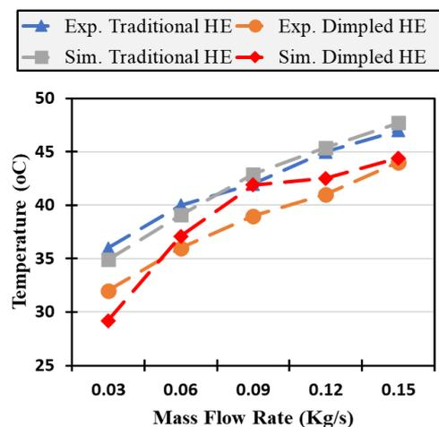
**Figure 21.** The experimental-simulation temperature recordings across the exit of the inner tube of the traditional vs. dimpled HE under all working condition of variant mass flow rates
