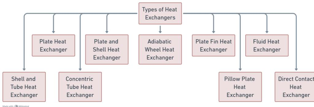
Figure 1. Typical heat exchangers design/construction classification
