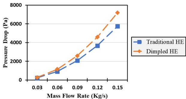
**Figure 23.** The simulation-based pressure drop calculations across the inner tube of the traditional vs. dimpled HE under all working condition of variant mass flow rates
