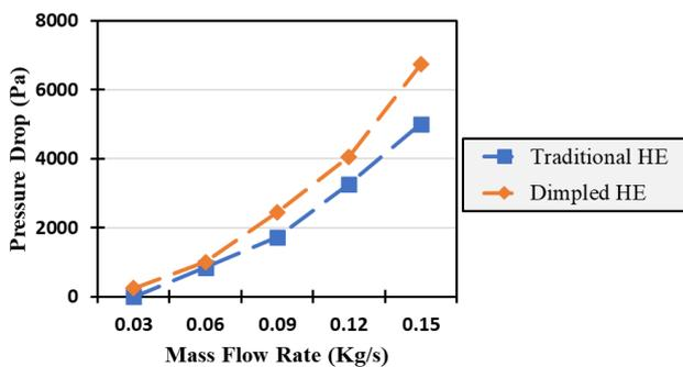
**Figure 22.** The experimental-based pressure drop calculations across the inner tube of the traditional vs. dimpled HE under all working condition of variant mass flow rates
