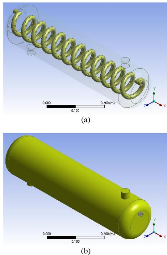
**Figure 7.** Helically-dimpled shell-and-tube HE of helical coils: (a) Helical copper tube, (b) Shell
