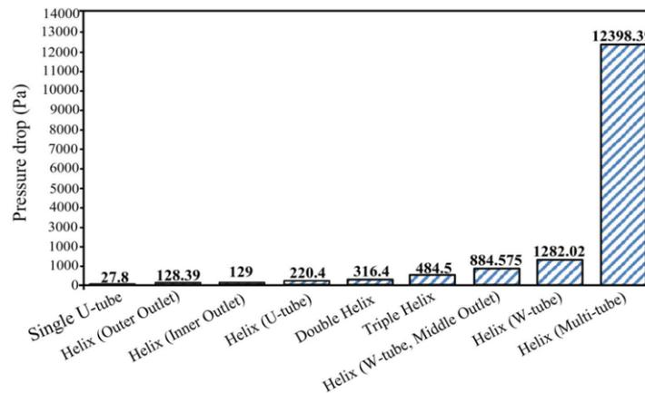
**Figure 3.** Pressure drop estimations of different helical tubes HEs [11]
