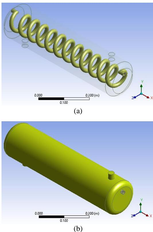
**Figure 6.** Traditional shell-and-tube of helical coils: (a) Helical copper tube, (b) Shell
