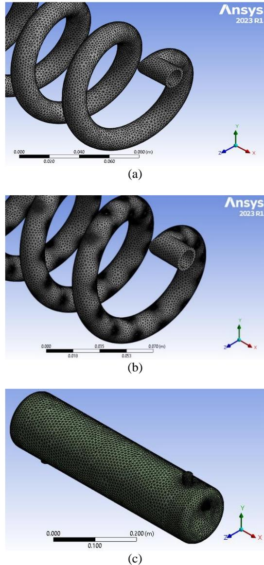
**Figure 9.** Mesh depiction: (a) Tube without dimples, (b) Inner tube with the dimple configuration, (c) Outer shell mesh for both cases
