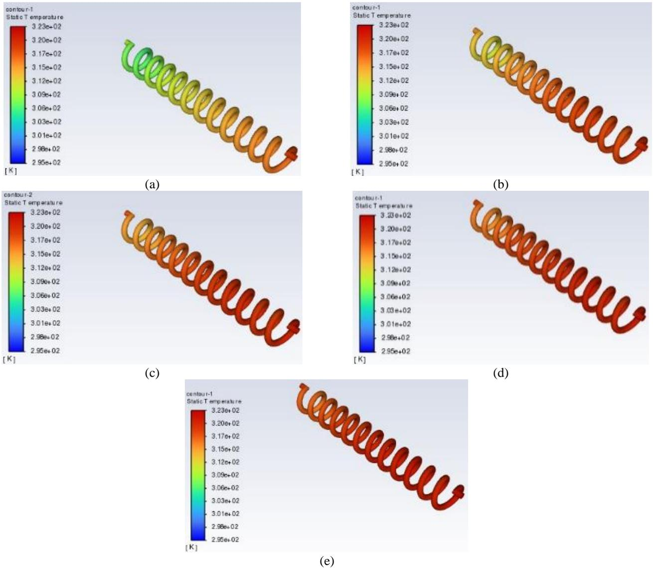
**Figure 14.** Traditional helical-tubed HE temperature profile across varying mass flow rates of: (a) 0.03 kg/s, (b) 0.06 kg/s, (c) 0.09 kg/s, (d) 0.12 kg/s, (e) 0.15 kg/s
