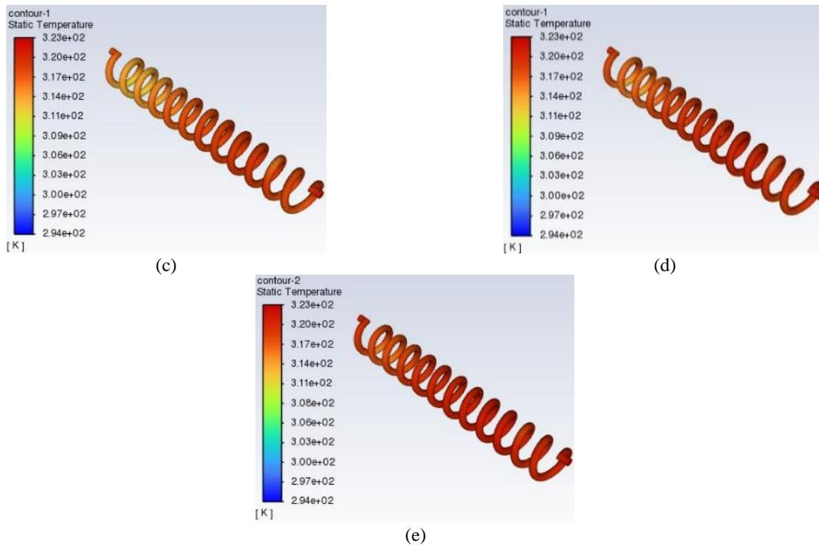
**Figure 15.** Dimpled helical-tubed HE temperature profile across varying mass flow rates of: (a) 0.03 kg/s, (b) 0.06 kg/s, (c) 0.09 kg/s, (d) 0.12 kg/s, (e) 0.15 kg/s
