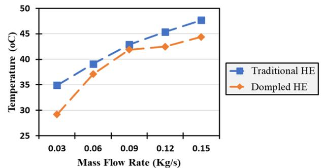
**Figure 20.** The simulation-based temperature recordings across the exit of the inner tube of the traditional vs. dimpled HE under all working condition of variant mass flow rates
