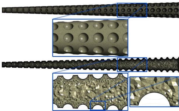
**Figure 4.** Comprehensive and cross-sectional mesh diagrams of a conical dimpled tube with a diameter ratio of 3 [24]
