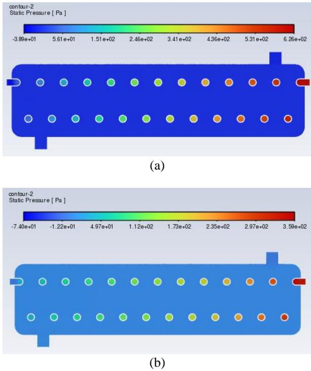
**Figure 18.** Cross-section for the pressure drop contours of the full HE under optimum working condition of 0.03 kg/s mass flow rate: (a) Normal HE, (b) Dimples HE
