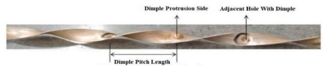
**Figure 5.** Helical smooth and dimpled configurations [30]
