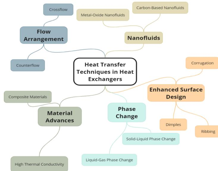
Figure 2. Heat transfer enhancement methodologies in heat exchangers
