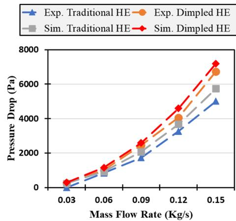
**Figure 24.** The experimental-simulation pressure drop calculations across the inner tube of the traditional vs. dimpled HE under all working condition of variant mass flow rates
