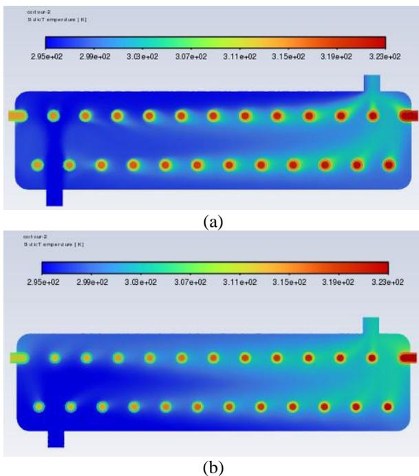
**Figure 16.** Cross-section for the temperature profile contours of the full HE under optimum working condition of 0.03 kg/s mass flow rate: (a) Normal HE, (b) Dimples HE
