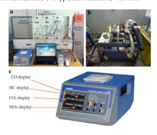
Figure 1. (a) Engine control unit, (b) engine block, (c) Gas analyzer device
